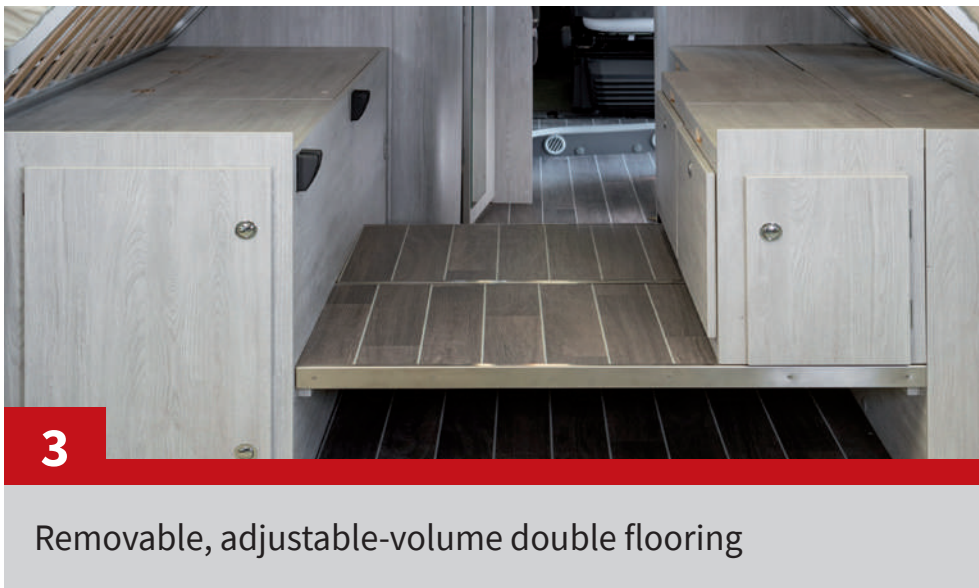
3 Removable, adjustable-volume double flooring
