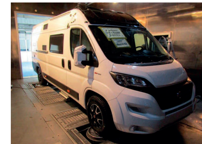
Vehicle in climatic chamber
