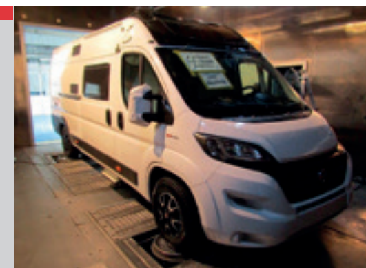
Vehicle in climatic chamber
